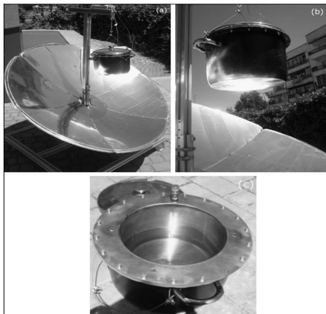
Fig. 2.2: (a) Cooker A in operation. (b) Focused sun on utensil. (c) Inner pot view with water[16]
